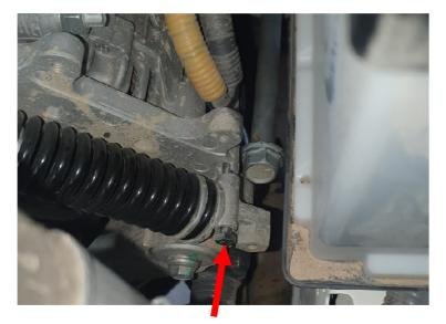
2. Place a 17mm spanner on the inner tensioner and pull it outward to allow you to install a pin (m6 bolt will work) into the upper inner tensioner hole.
