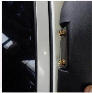
21. Remove the snorkel and remove the mounting bracket from the snorkel body. Hold the mounting bracket back into the position marked in the previous steps and mark the hole positions.
