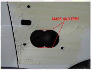
12. Using the Pneumatic hacksaw cut between the 2 holes top and bottom horizontally to make an oval.
