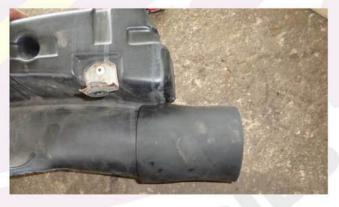
30. Remove the original foam seal from the air-box elbow inside the wheel arch.
