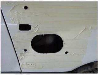
13. Using the step drill, drill a few larger holes in the centre of the new indicator position. This will allow you to start to cut the shape out with the pneumatic hacksaw.
