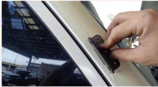
22. Centre punch then pilot drill the holes, and then drill to 7.5mm It is a good idea when doing this to drill through a block of wood or equivalent spacer so that only about 5mm of the drill tip sticks out so you do not drill through the interior or air bags.
