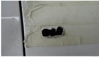
14. Using the pneumatic hacksaw carefully cut out the new indicator position.
