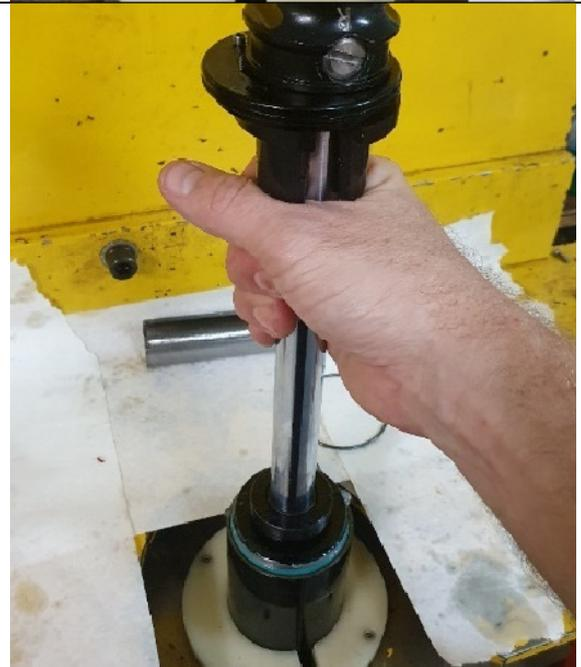
8. When the main piston is almost out of the shock, remove the top attachment from the machine if using machine, and then slowly pull the piston up by hand, with your fingers around the wear band so it doesn't fall into the shock
