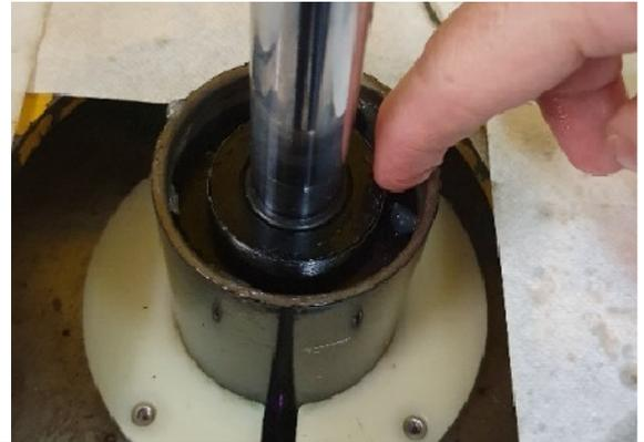
7. Pull up the rod and seal head assembly together, wiggling as you go and remove from shock. This can also be quite difficult and may require you to pull it up, push it back down, regrease the circlip groove and try again or hold the rod end and shaft in softjaws vice while you tap the body down with a rubber mallet.
