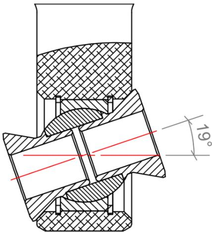
HIGH ANGULAR TRAVEL APPLICATIONS - O-RINGS REMOVED, HI-ANGLE SPACERS FITTED. MAX APPROX. 19°
