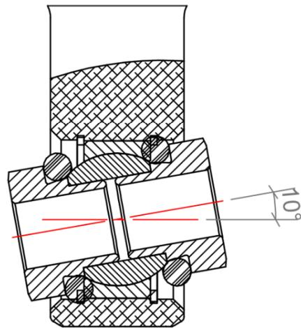
LOW ANGULAR TRAVEL APPLICATIONS - STRAIGHT MISALIGN SPACERS & O-RINGS FITTED. MAX APPROX. 10°
