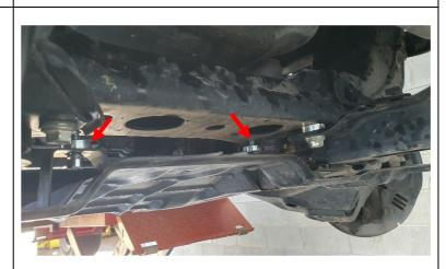
9. Reinstall the bash plates using the OEM hardware.
