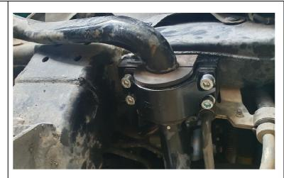
7. NOTE: If installing a diff drop kit as well, this will typically be supplied with slightly longer bash plate spacers to allow clearance of the lower diff position. If this is the case use those spacers and bolts supplied instead and skip the remaining steps.
