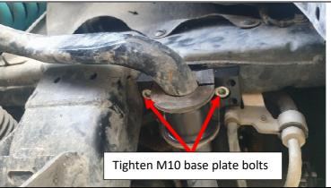
6. Re-Install the D bracket with M8 x 1.25 bolts with spring washer and flat washer to Base plate and tighten.
