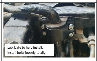
Carefully remove the D-bracket installed in step 4 and tighten the M10 bolts in the base plate installed in step 2.
