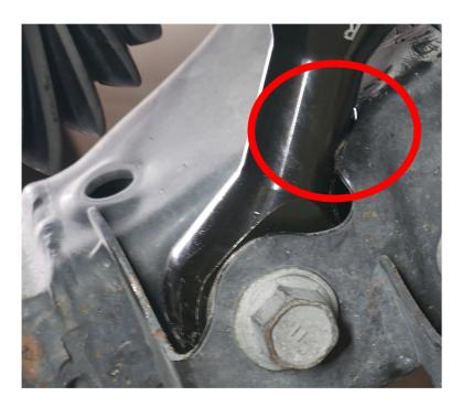
NOTE: For proper fitment, the inside of the lower control arm shock mount will need to be trimmed
