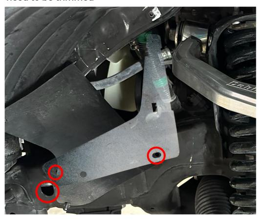
Remove the plastic chassis cover behind the body mount, remove the two lower clips holding the splash guard. Use both captive nuts and insert them through the oval hole. Install the bolts through the holes that were used to hold the splash guard.
