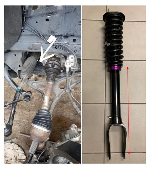
BOTH SIDES: To install please remove the top ball joint, the sway bar link, tie rod end and loosen ABS LINES.
