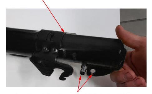
CHECK IF ORIGINAL BOLT IS ABOVE FLANGE OR THROUGH HOLE. FIT THE SAME AS ORIGINAL
