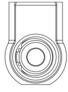
HIGH ANGULAR TRAVEL APPLICATIONS - O-RINGS REMOVED, HI-ANGLE SPACERS FITTED. MAX APPROX. 19° ENSURE CIRCLIP OPENING IS IN A HORIZONTAL POSITION SO THAT IT DOESN'T NOT BIND ON THE SPACERS
