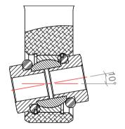
LOW ANGULAR TRAVEL APPLICATIONS - STRAIGHT MISALIGN SPACERS & O-RINGS FITTED. MAX APPROX. 10°
