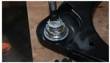
3. **Using 40mm ID and 68mm ID press cups**. DO NOT PRESS ON THE END OF THE THREAD UNDER ANY CIRCUMSTANCES. Ensuring you press from the housing to prevent damage.
